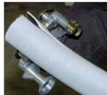
Teeth Gripping and Pulling Off Laminate Layer.
